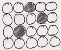
Disordered Substitutional Solid Solution
