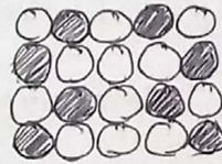
Ordered Substitutional Solid Solution.
