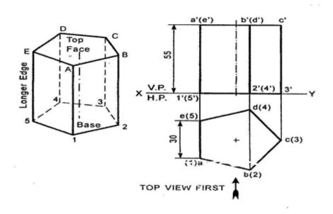
Solved Problem – 4: Draw the projections of a hexagonal prism of side of base 25 mm and height 50 mm resting with its base on HP such that one of its rectangular faces is perpendicular to VP.
