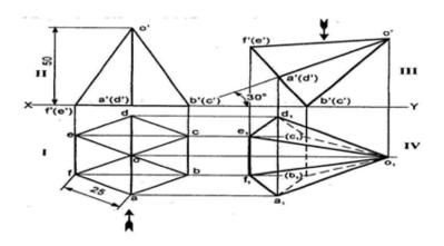
Solved Problems-17: Draw the projections of a pentagonal pyramid of base 25 mm side and axis 60 mm long when it is lying on HP on one of its base edges, such that the axis is parallel to VP and inclined at 30° to HP.
