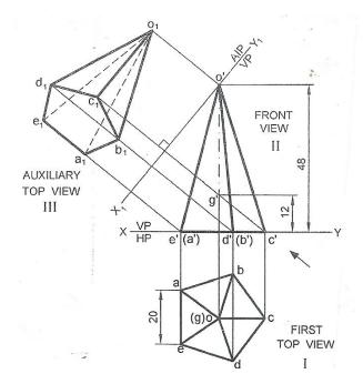
2. Draw the top view such that the line joining c and the center of gravity (g) of the pyramid parallel to XY. Project front view as shown.
