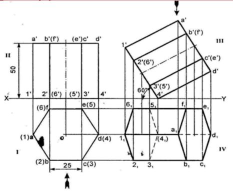
Solved Problems 23: A pentagonal pyramid side of base 20 mm and axis 45 mm long rests with one of its corners on HP such that the base is inclined at an angle of 60° to HP and one side of base is perpendicular to VP. Draw its projections.
