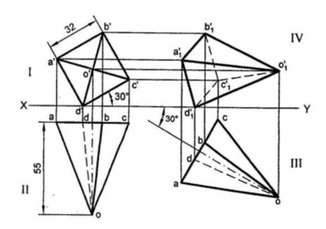
Solved Problems– 29: A square pyramid of base end 40 mm and axis 60 mm is lying on VP on one of its triangular faces with the plane containing the axis parallel to HP and 30 mm above it. Draw the projections of the pyramid.
