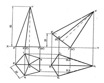
Solved Problems - 20: A hexagonal pyramid of 26 mm side of base and 70 mm height rests on HP on one of its base edges such that the triangular face containing the resting edge is perpendicular to both HP and VP. Draw its projections.
