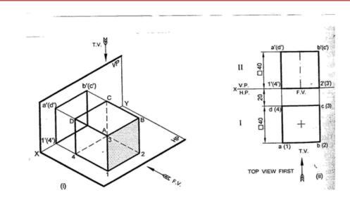
Solved Problem – 2: A cube of 40 mm side rests with one of its square faces on HP such that one of it vertical faces is perpendicular to VP. Draw its projections. The nearest edge parallel to VP is 5 mm in front of it.
