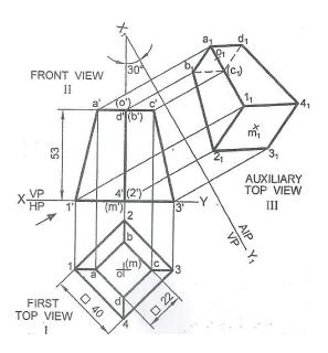
Solved Problems – 35: An octahedron of 35mm side lies with one of its faces on HP and an edge of that face makes an angle of 90° with VP. Draw its projection.
