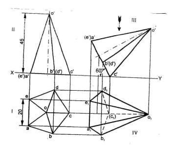
Solved Problems- 24: Draw the projections of cone, base 30 mm diameter and axis 50 mm long, resting on HP on a point of its base circle with the axis making an angle of 45° with HP and parallel to VP.
