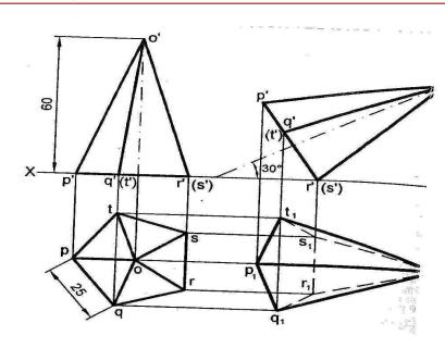
Solved Problems- 18: A tetrahedron of 40 mm side rests with one of its edges on HP and perpendicular to VP. The triangular face containing that edge is inclined at 30° to HP. Draw its projection.
