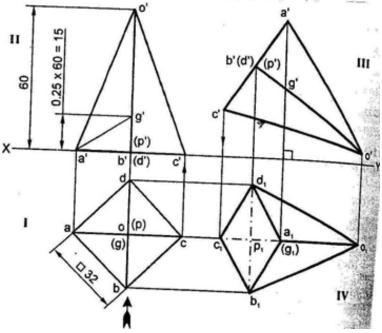
Solved Problems-27: A cone of diameter 40 mm and height 60 mm is freely suspended from one of its base points such that the axis is parallel to VP. Draw its front and top views.
